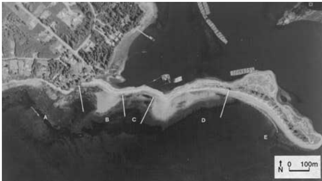
FIGURE 3: A vertical air photo of Whiffin Spit at the entrance to Sooke Harbour. Some portions of the spit include both a gravel beach and a sand & gravel flat (Units B,D) whereas other portions are just gravel beaches (Units C,E).
