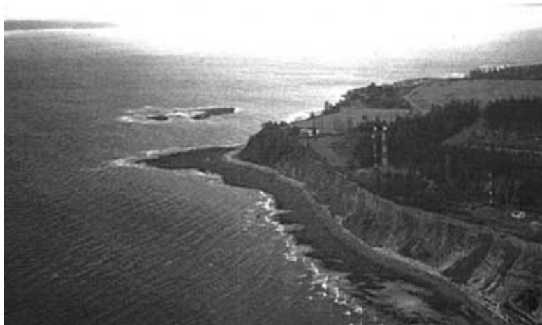
FIGURE A.1: Oblique aerial photo of the eroding cliffs at Cape Lazo near Comox (Denman Island in background).The cliffs are cut into unconsolidated marine sediments and include a discontinuous talus apron. The beach is gravel, primarily pebble/cobble and a wide beach terrace with a boulder/cobble armour lies seaward of the beach.
